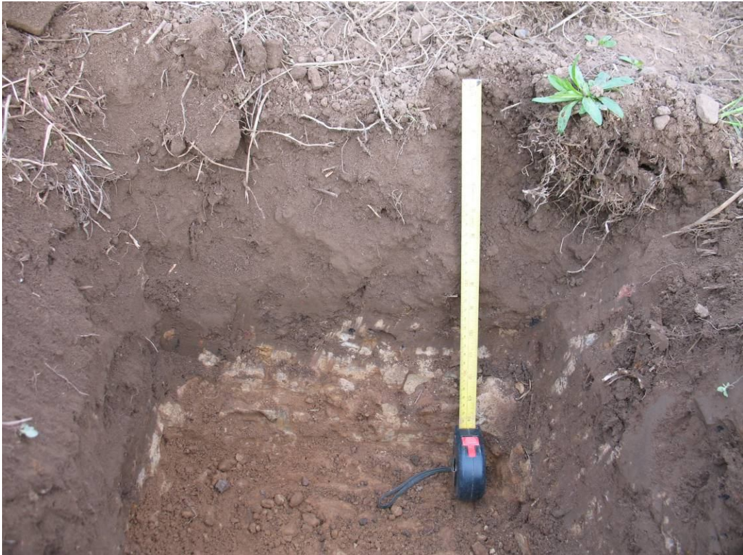
Plate 2: Permeable sandy loam soil on stone rock at shallow depth (25cm). Drought restricts grade to 3b.
