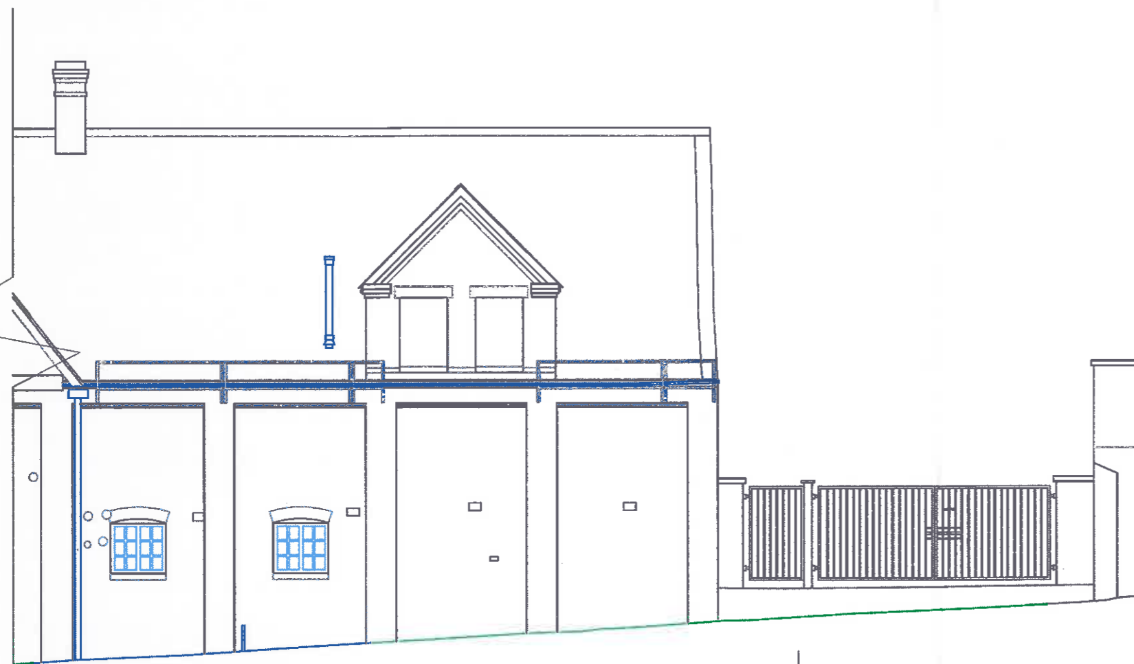
EXISTING FRONT ELEVATION
